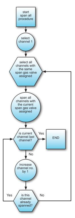
Fig. 7-5: Span All Calibration Procedure Flow Diagram
